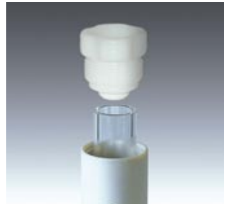
The components of the Q-20 vessels: TFM cover, high-purity quartz vessel, and safety shield with built-in safety valve.
